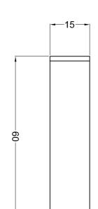
Flatness End Chamfers: Polished Surfaces "A": Cosmetic (S/D): Long Edge Chamfers Fine Polish ≤ 0.5mm x 45° ≤ 3\ @ 633nm 60/40 Minimum
