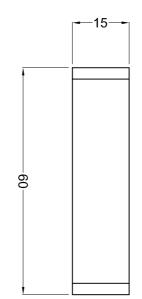
Flatness: Polished Surfaces "A": Cosmetic (S/D) Long Edge Chamfers Fine Polish ≤ 0.5mm x 45° ≤ 3\ @ 633nm 60/40 Minimum
